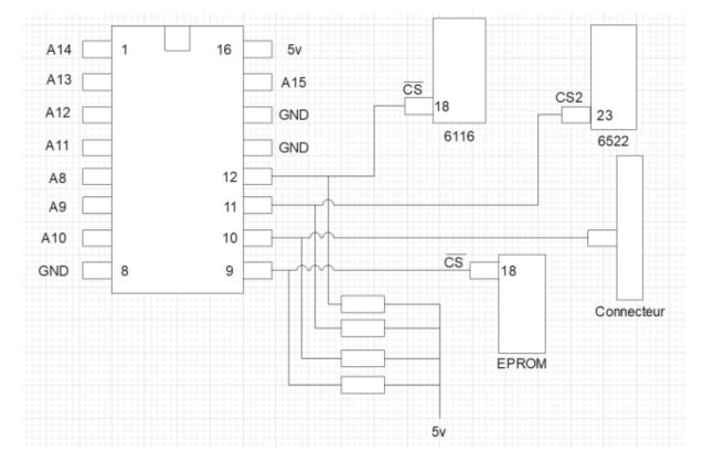
With this schematic we can determine the role of each output pin
